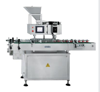
CVC tablet/Capsule Counter has a simple and reliable design: tablets or capsules loaded from a stainless steel hopper are arranged by a rotary disc, and detected by optical fiber sensors as they are counted and filled into the container.
