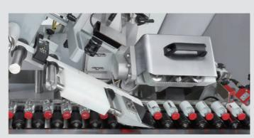
\* The tension adjustable wrap belt can tolerate differentials of each ampule and prevents breakage under high speed operation. Flip design enables easy cleaning.
