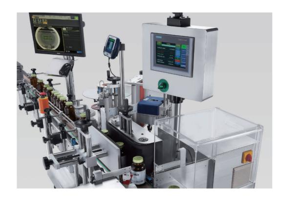
Enjoy peace of mind with a CVC SelfSet™ labeler. Simply place a container on the conveyor and with just a press of a button, all speed adjustments are instantly calculated and synchronized for the start of your next production run. Your automatic labeler setup has never been so easy!
