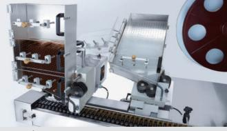
\* Ampoule/ Vial loading cassette can be refilled while the machine is running (Option)
