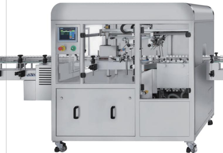
The CVC 1102-400/ CVC 1102-600 Bottle Air Rinser are equipped with powerful clean air jet and vacuum suction which are combined with 180-degree inversion of bottle at speeds of up to 80-120 bottles per minute. The CVC 1102 series Automatic Bottle Air Rinser are the ideal solution for bottle packaging lines to achieve cGMP compliance.
