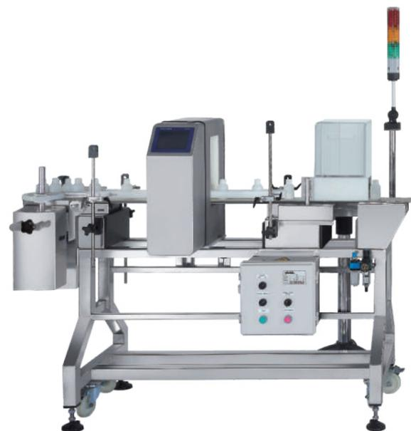
The CVC 1430SS utilise a low power, high frequency, magnetic field coil system that has the ability to sense minute disturbances created by metal particles. A metal particle passing through the aperture of the detector creates changes in the magnetic field inside the detector.
