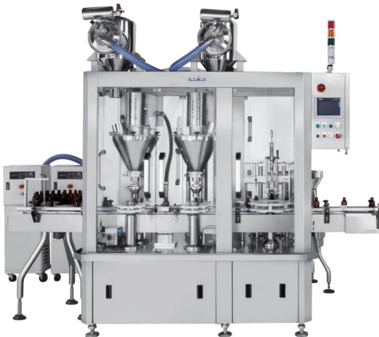
Designed for metering and filling various kinds of powder and granular products into bottles/cans, such as, medicine powder, food powder and chemical powder... etc.
