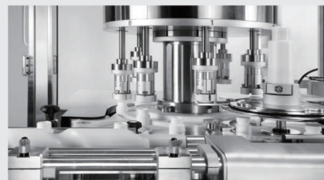
• Capping head up/down and rotation are individually driven by advanced Linmot liner motors and servo motors.
