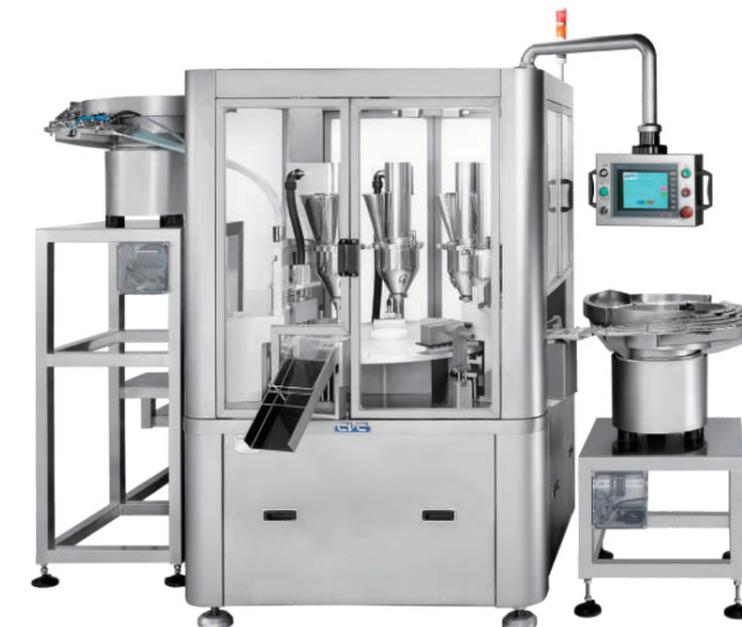
The monoblock auger filling system consists of four stations for plastic bottle sorting/ feeding, powder filling, plugging and filled product discharging.
