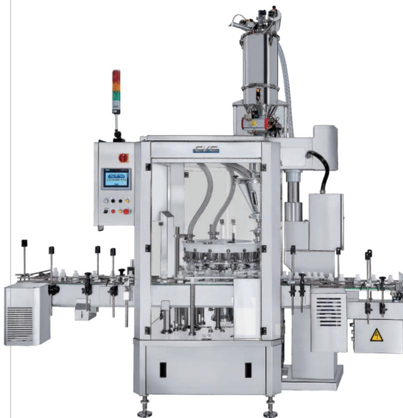
The CVC 6088-R16/ 6088-2R24 Automatic Rotary Powder Filling Machines are designed to fill powder products into containers provided to its infeed conveyor and transported through its rotary continuous motion mechanism. The Powder dosing uses servo motor driven auger dosing system for accuracy volume.
