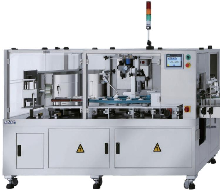
The CVC 1266 Bottle Unscrambler is designed to automatically feed bottles from a bin and place them upright onto a conveyor at speeds of up to 250-280 bottles per minute. The CVC 1266 is built on a Siemens control system including a HMI panel. Options include ionized air rinse with vacuum, fallen bottle sensor with return to bin, low level hopper sensor, tower lamp, and static eliminator bar. No change parts are required.
