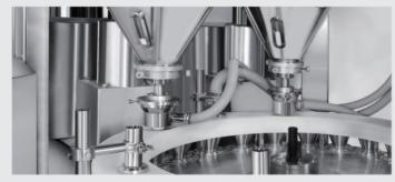
· CVC 6088-2R24: Double head auger powder filling & 24 filling station
