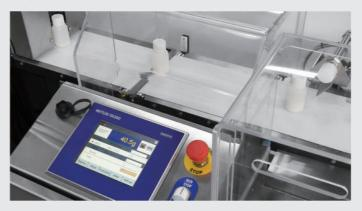
The CVC 1430SS utilise a low power, high frequency, magnetic field coil system that has the ability to sense minute disturbances created by metal particles. A metal particle passing through the aperture of the detector creates changes in the magnetic field inside the detector.
