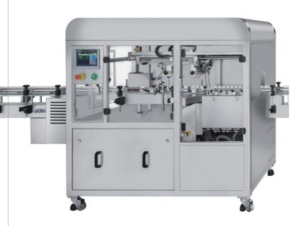
The CVC 1102-400/ CVC 1102-600 Bottle Air Rinser are equipped with powerful clean air jet and vacuum suction which are combined with 180-degree inversion of bottle at speeds of up to 80-120 bottles per minute. The CVC 1102 series Automatic Bottle Air Rinser are the ideal solution for bottle packaging lines to achieve cGMP compliance.
