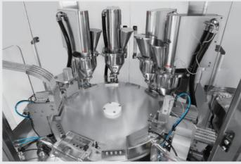
• The central starwheel driven by cam system can stabilize the transmission of small plug/ cap, and offers precise operation.
