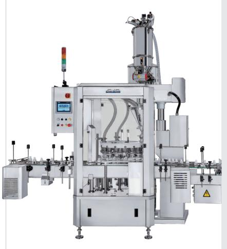
The CVC 6088-R16/ 6088-2R24 Automatic Rotary Powder Filling Machines are designed to fill powder products into containers provided to its infeed conveyor and transported through its rotary continuous motion mechanism. The Powder dosing uses servo motor driven auger dosing system for accuracy volume.
