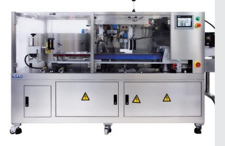
The CVC 1266 Bottle Unscrambler is designed to automatically feed bottles from a bin and place them upright onto a conveyor at speeds of up to 250-280 bottles per minute. The CVC 1266 is built on a Siemens control system including a HMI panel. Options include ionized air rinse with vacuum, fallen bottle sensor with return to bin, low level hopper sensor, tower lamp, and static eliminator bar. No change parts are required.
