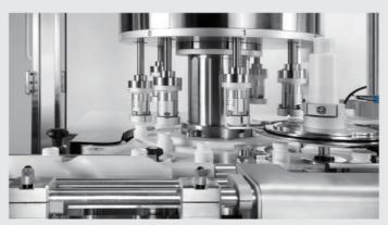
• Capping head up/down and rotation are individually driven by advanced Linmot liner motors and servo motors.
