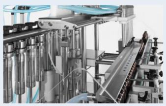
Shut-Off Nozzles and Drip Tray: Shut-off nozzles are strongly recommend for liquid with low viscosity
