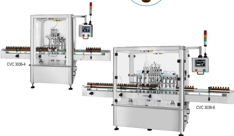
The CVC 3036 ser. linear type liquid filler is designed for bottle filling of general liquids widely used in pharmaceutical, nutraceutical, food, chemical and cosmetics industries.
