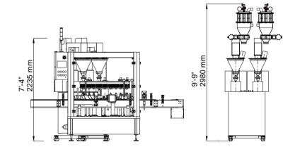
The dimensions shown are for standard machine with optional infeed and outfeed conveyor. Optional conveyor for bottle transporation is available upon request. This machine with an optional conveyor can run independently or be integrated into an automated packaging line. All CVC equipment is covered by a one-year parts warranty. Full Warranty details are included in our equipment proposals or can be found on our website.
