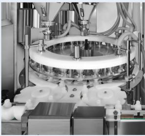
• Double head auger powder filling & 24 filling stations.
