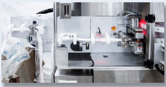
Cotton pre-feed device features smooth and non-stop cotton feeding.
