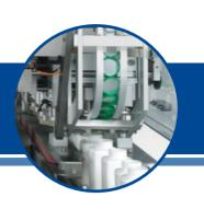
The CVC 1206 Capper is a very flexible machine designed to apply and tighten screw-on caps onto containers at rates of up to 140 bottles per minute. The CVC 1206 is Siemens PLC controlled. The system is designed with three pairs of capping spindles. Options include tower lamp, hopper level control, cap inspection (level cap, foil seal, and no cap), reject, and reject verification.
